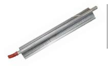
Electric heater consisting of finned aluminum elements, ensuring low surface temperature and deleting the air ionization problems. The optional is installed downstream the main cooling coil. In electric heaters with three working steps the activation is binary type. Components:
