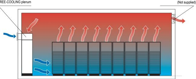
The plenums have same technical characteristics and base dimensions of the machine cabinet. The optional allow to obtain free-cooling by direct ambient air intake into the room. The dampers are proportionally managed by the microprocessor control, that regulates the quantity of the ambient air to put in the room according to the set-point.
